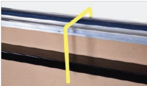
Safety lock secures stage in position while moving
